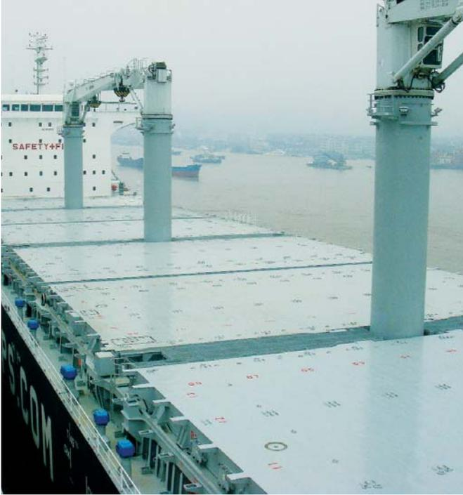
After an absence from the Chinese market of more than fifteen years, TTS piggy-back hatch covers are making a comeback, featuring in the delivery of a 50,000 dwt multi-purpose vessel from Zhejiang Shipping Group Zhoushan Wuzhou Ship Building and Repairing Co Ltd to German shipowner NSC Schifffahrtsgesellschaft.
